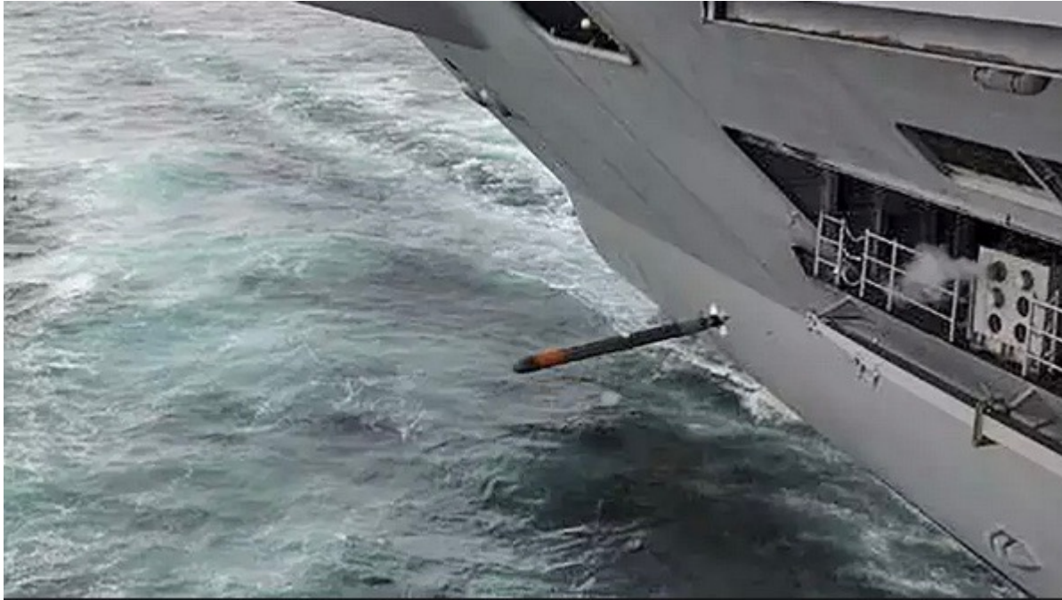
Antytorpeda systemu ATTDS. Fot. US Navy
